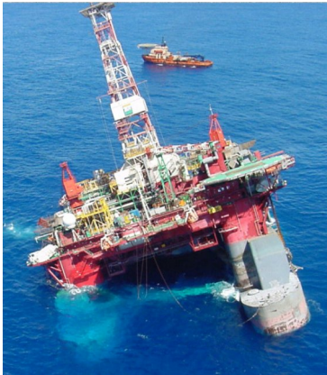
Figure 26- Sstab evaluation of flooding using measured drafts.
