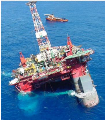
Figure 26- Sstab evaluation of flooding using measured drafts.
